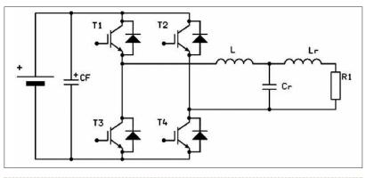
Figure 2: Voltage source inverter with inductive coupling (ZVS mode) and parallel resonant circuit
