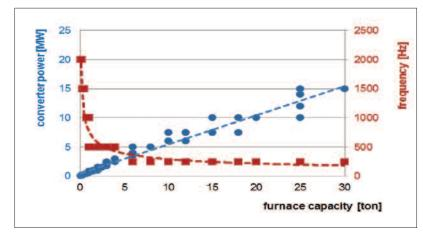
Figure 1: Typical converter power and operating frequency as a function of induction heating furnace capacities a resonant inverter.
