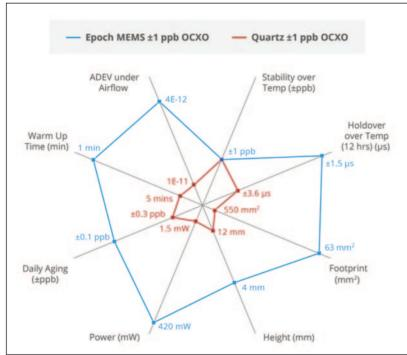
battery life in portable and IoT devices. In our increasingly wireless and mobile world, the low power consumption of MEMS-based timing solutions is a significant advantage.
