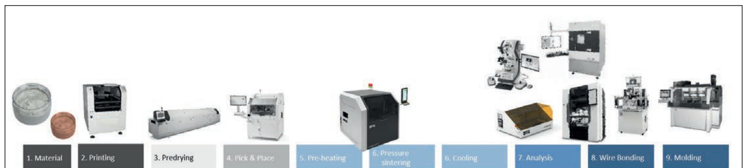
Figure 2 – Equipment used in the fabrication of a power electronics component/module requiring die to be sintered to the substrate. Not shown, but a recent industry development is the use of a foil with a similar composition to a paste. Printing and pre-drying can be skipped, but the foil is expensive and requires special handling. The technique is more for R&D work than volume production.
