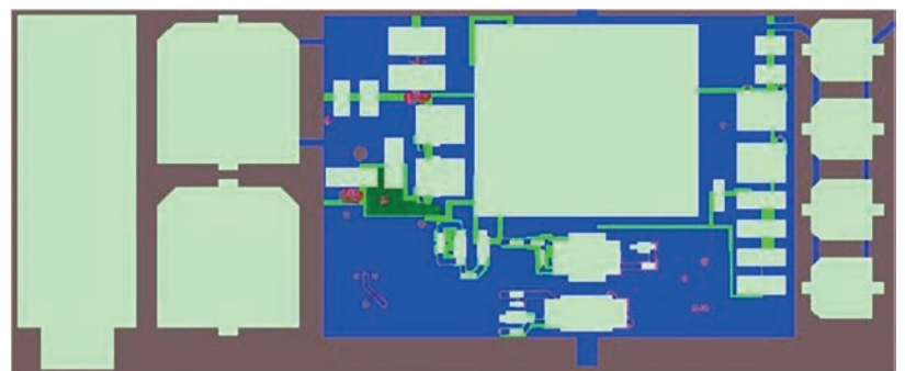
Figure 2: The input-side holdup design option measures 116.84 x 47mm.
