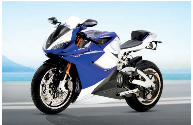
Figure 2 Minimally, electric motorcycles need to deliver 100 miles at 70 miles an hour per charge. Today Lightning's bikes range more than 170 miles/charge with the capacity to recharge to 80 percent in 10 minutes.
