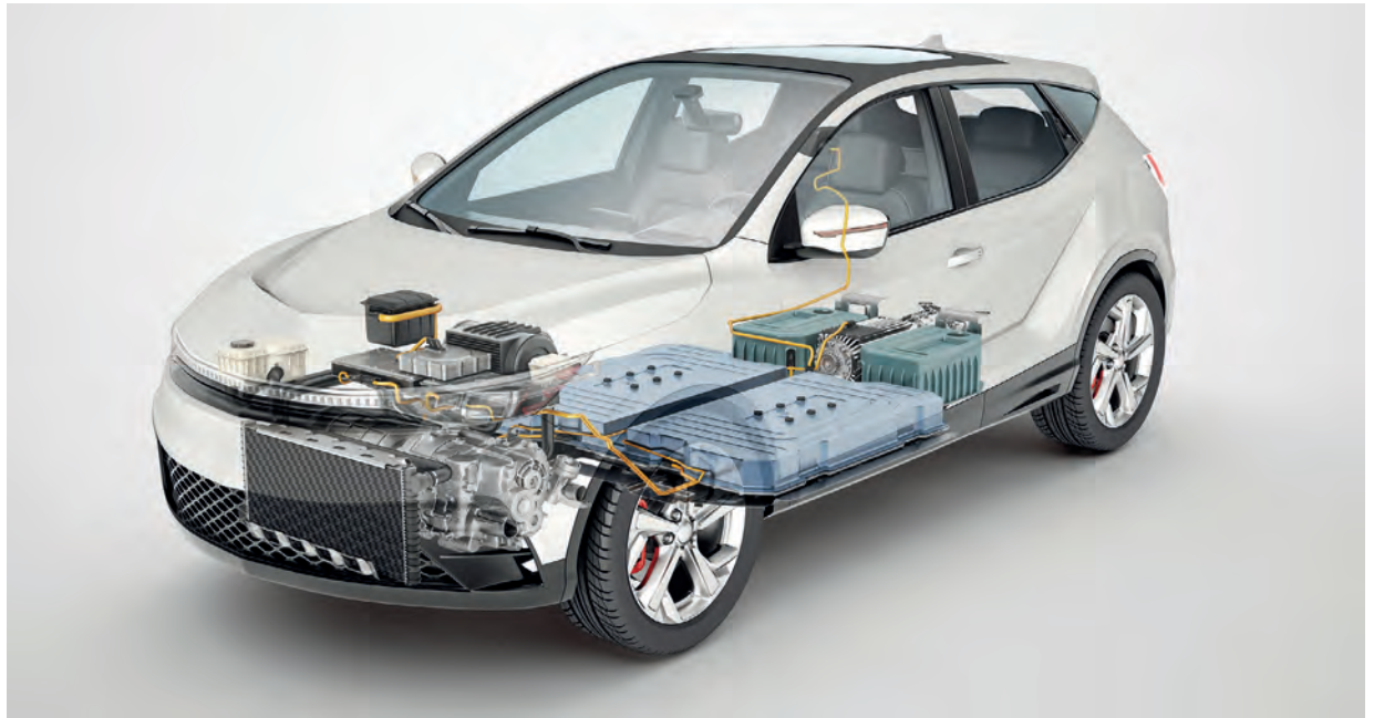
Figure 2: Conventional EV design has to accommodate battery packs and the driver train.
