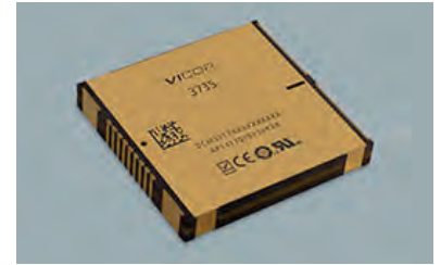
Figure 5: The DCM3735 is a non-isolated, regulated DC-DC converter with an input range of 35-58V. It offers constant current operation for battery charging, comes in a compact package (36.6 x 35.4 x 7.4mm) and can be used in array.
