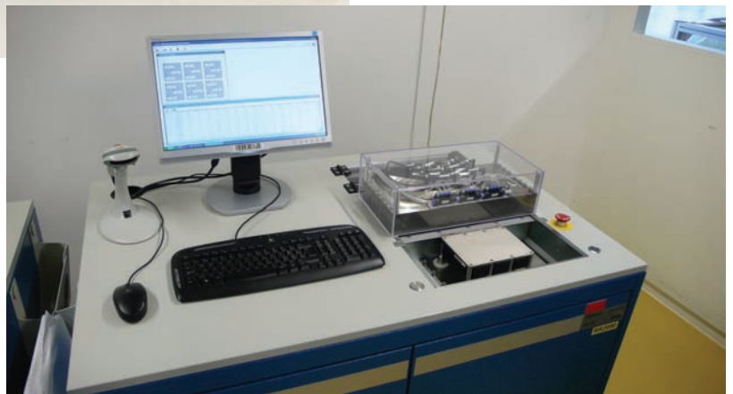
Figure 2: Baseplate flatness test system
