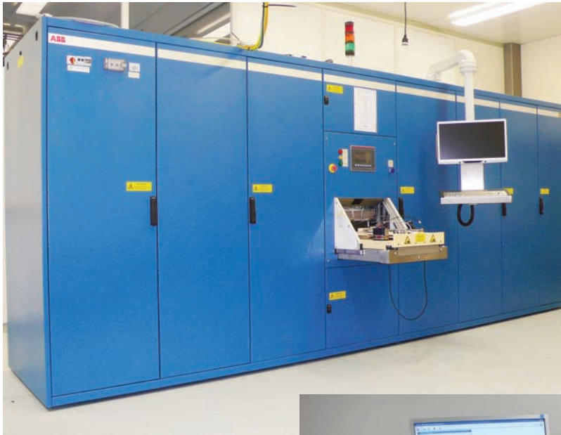
ABOVE Figure 1: Static and dynamic test system for thyristors and diodes
