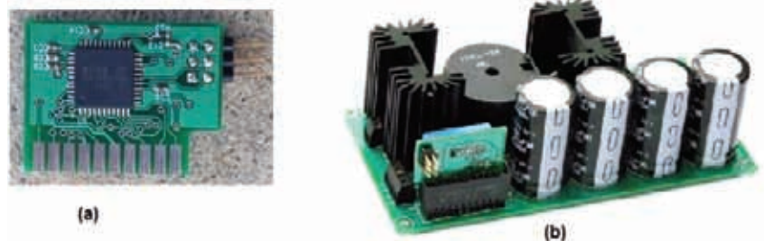
Figure 5: MCU module (a) and main power board with MCU module (b)
